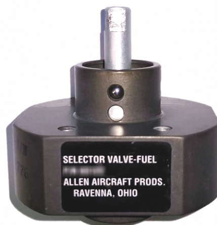
Figure 1 Fuel Selector Valve, Piper P/N 491-947
