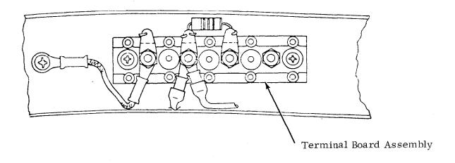
FIGURE 2 - Terminal Board After Modification
