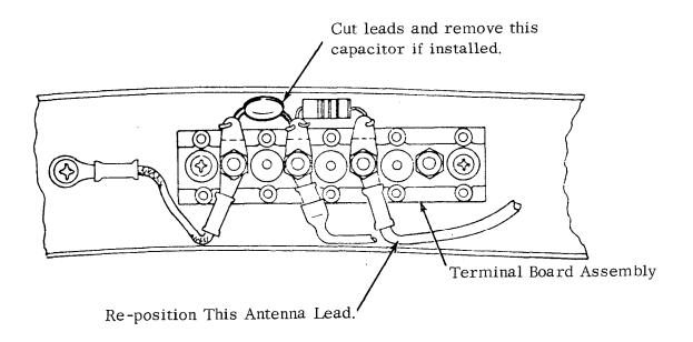
FIGURE 1 - Terminal Board Prior to Modification
