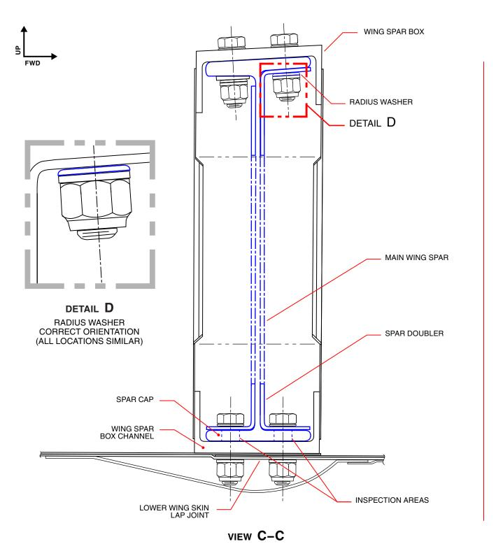
WING SPAR CROSS SECTION SHOWN AS INSTALLED IN WING SPAR BOX
