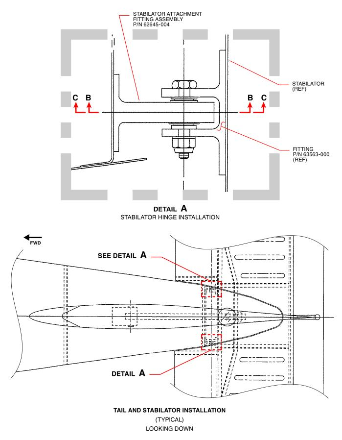
Figure 1, Sheet 1 of 3 Stabilator Attach Fitting Assemblies
