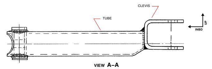
STABILATOR IDLER ARM, P/N 67066-000 CORRECT ORIENTATION AS INSTALLED LOOKING AFT
