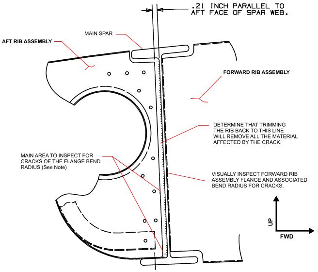
NOTE: Applicable to the initial 50 hour inspection and 500 hour recurring inspection. Not applicable to the recurring 100 hour inspection.
