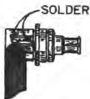
FIGURE 2-2 ANTENNA CABLE ASSEMBLY (DWG. NO. 696-6003-00)
