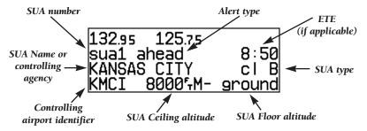
The 'SUA number' field displays which SUA you are viewing (you may be alerted to up to nine SUAs). SUAs are ranked with 'sual' being the highest priority, and 'sua9' being the lowest priority from your current position. The 'SUA alert' field displays the corresponding alert message for this SUA, such as 'near', 'near & ahead', etc. (see page 58). The ETE (estimated time en route), located at the top right of the page, will only be displayed if you are projected to enter the airspace.
