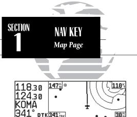
On the map page the active and standby communication frequencies are in the upper left corner of the page. The active frequency is on top.
