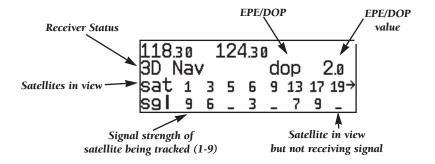
The top lines of the status page display active and standby frequencies, followed by the receiver status and the current position accuracy in DOP or EPE. The default setting is DOP. The following functions may be displayed in the DOP/EPE field:
