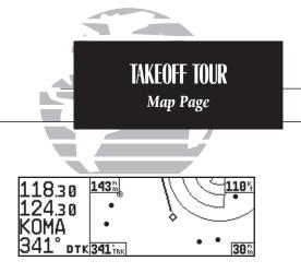
The map display may be oriented along your ground track (track up), course (desired track up) or fixed at north up. Desired track up or north up settings show your present position with a diamond symbol instead of the airplane symbol.
