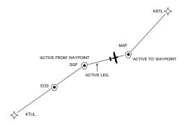
As you pass each waypoint in the route, the GNC 300XIs automatic leg sequencing and turn anticipation features will automatically select the next waypoint as the 'active to' waypoint and provide smooth steering guidance around the turn. If you are not currently navigating a particular route leg (e.g., your starting position is not a route waypoint), the unit will select the appropriate leg as the active route segment.
