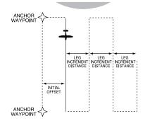
The map page will show the active leg of the search and rescue pattern as a solid line with the anchor waypoints joined together by a dashed line.
