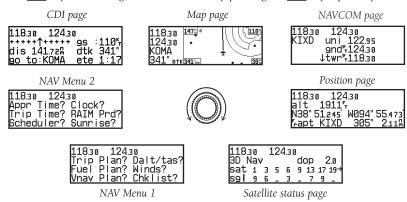
The **CDI**, **map**, **NAVCOM** and **position** pages are the primary pages used during in-flight navigation, while the nav menu and status pages offer access to planning, calculation and status functions. Note that rotating the outer knob clockwise will continuously cycle through all the navigation pages, whereas turning the knob counterclockwise will stop the page selection sequence at the CDI page.
