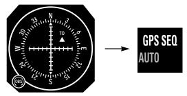
Always set the desired course on the HSI (OBS) BEFORE returning the GPS SEQ switch to the 'AUTO' position.
