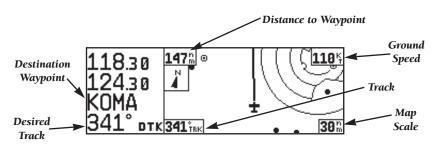
The **data fields** on the map page indicate distance to destination waypoint, desired track, ground track, ground speed and map scale. The destination waypoint name and desired track appear on the left side of the page, below the communication frequencies. The other data fields are located at the corners of the map display as shown in the illustration above, and may be removed by pressing CLR.
