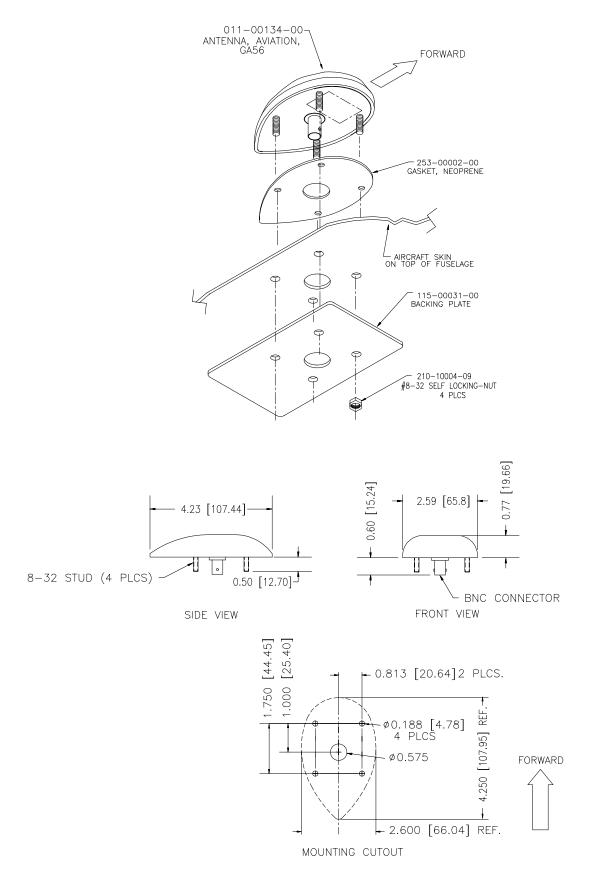
FIG 3-1 STUD MOUNT GA 56 ANTENNA INSTALLATION
