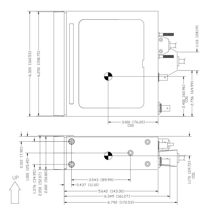
FIGURE 3-4 AVIATION RACK DIMENSIONS
