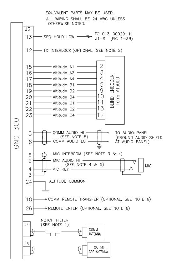
FIGURE 1-3C INTERCONNECT SCHEMATIC
