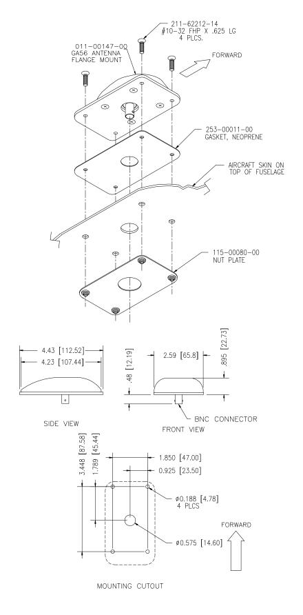
FIGURE 3-2 FLANGE MOUNT GA 56 ANTENNA INSTALLATION
