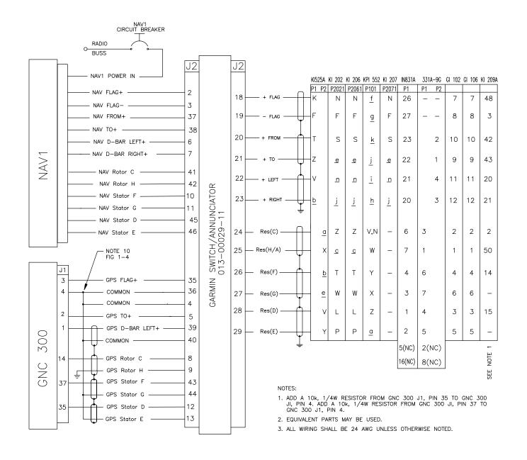
FIGURE 1-3A INTERCONNECT SCHEMATIC
