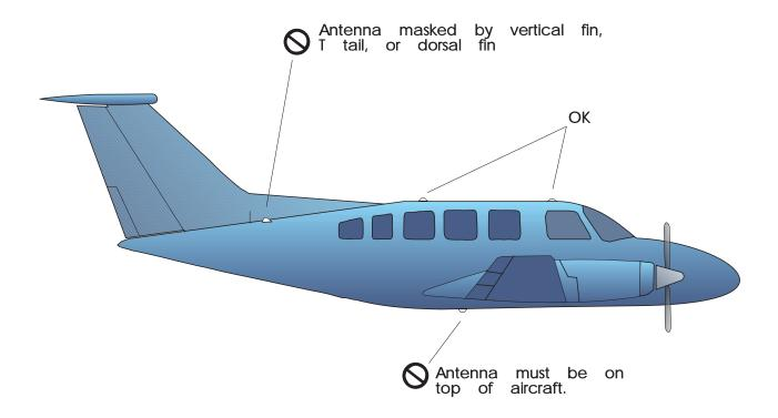
FIG 2-1 GPS ANTENNA INSTALLATION CONSIDERATIONS
