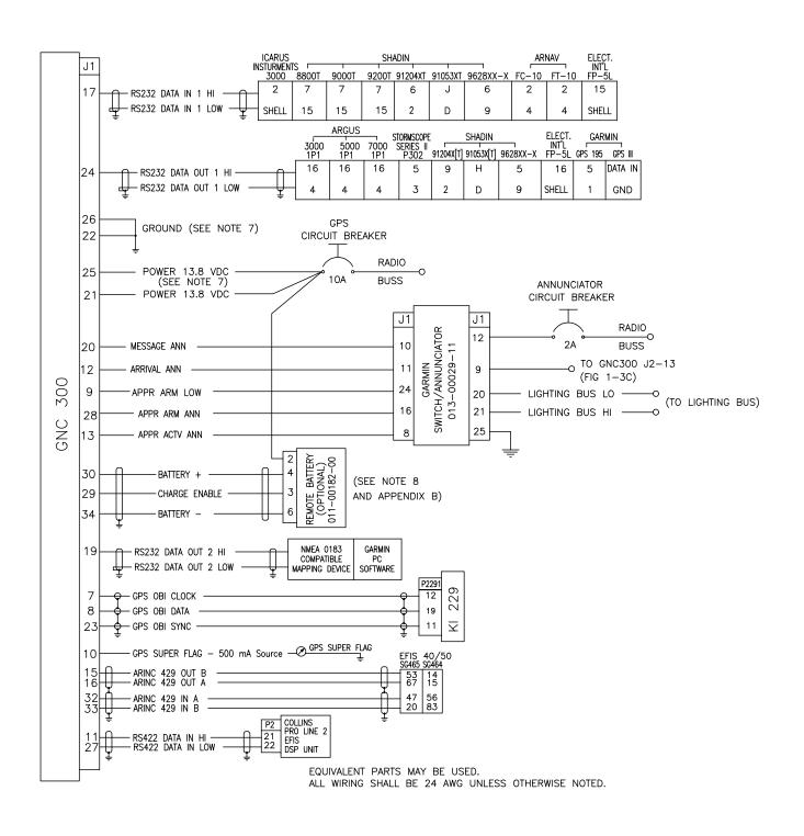
FIGURE 1-3B INTERCONNECT SCHEMATIC
