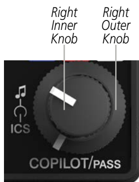
Right Knob - Copilot and Passenger Volume Controls
