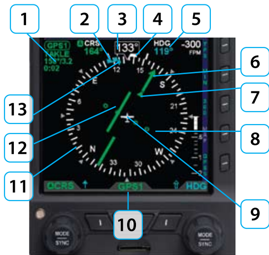
Figure 4-32 Horizontal Situation Indicator
