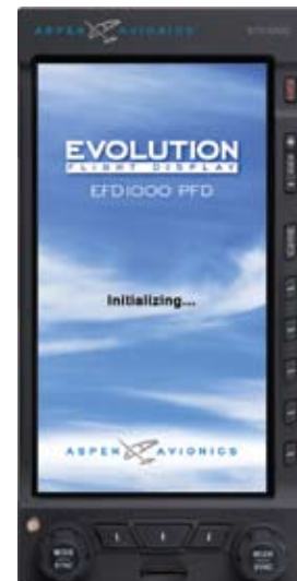
Figure 3-2 EFD1000 PFD Initializing
