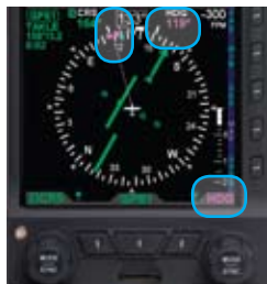
Figure 2-4 Activating the HDG field to edit
