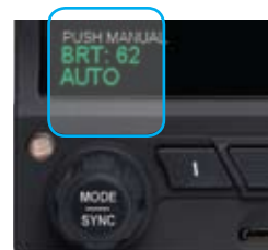
Figure 5-25 Display Brightness in BRT AUTO Mode
