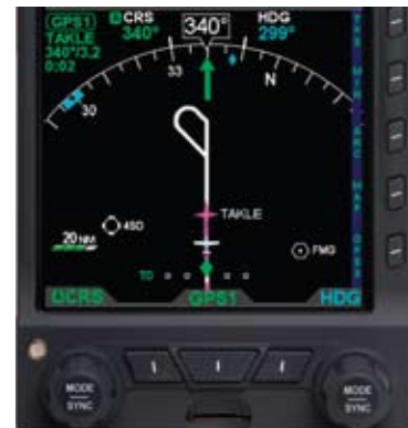
Figure 3-34 ARC Mode Showing Procedure Turn, GPSS Enabled
