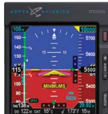
Figure 2-32 Instrument Approach Indications
