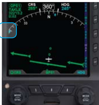
Figure 4-76 Selected Heading Bug Outside of ARC Range
