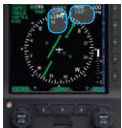
Figure 2-6 HDG field updated and inactive
