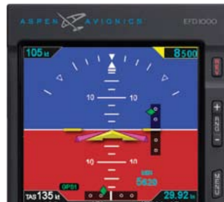
Figure 4-10 Airspeed Tape Disabled
