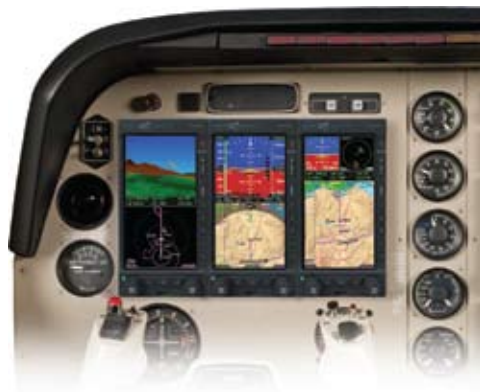
Figure 1-4 Three-tube system: PFD & dual MFDs
