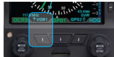
Figure 4-73 173 Single-Line Bearing Pointer and Button
