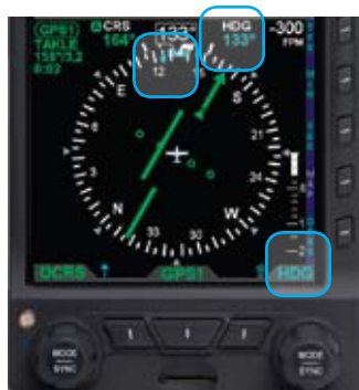
Figure 3-10 Heading Field Disabled
