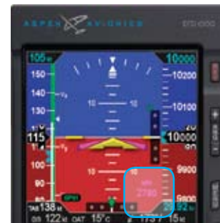
Figure 4-24 MIN Field Enabled
