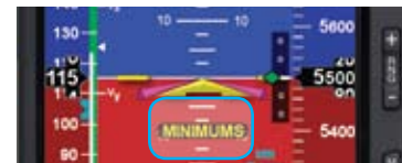
Figure 4-26 Minimums Alert Active
