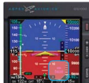
Figure 4-25 New MIN Setting
