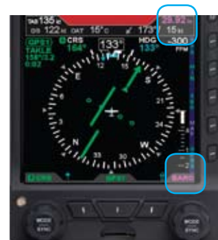
Figure 3-7 BARO Field Enabled
