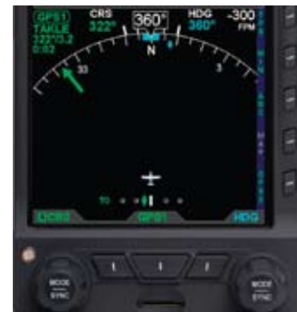
Figure 4-40 ARC Compass Mode
