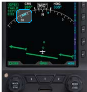
Figure 4-75 Selected Heading Bug and Numerical Display
