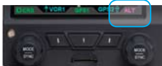
Figure 3-19 Altitude Field Enabled
