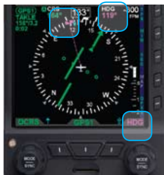
Figure 3-9 Heading Field Enabled
