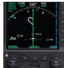
Figure 4-34 ARC HSI Compass Mode
