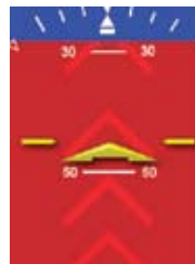
Figure 4-3 Pitch Markings - Large Pitch Up
