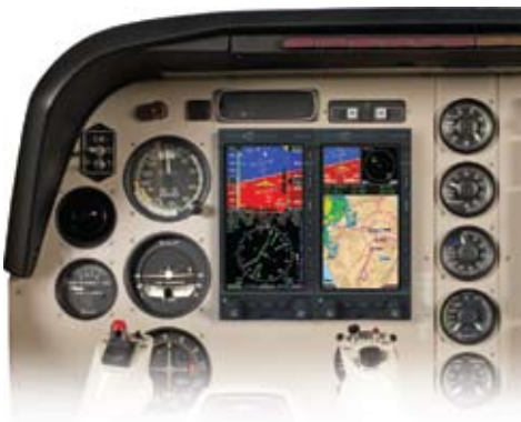
Figure 1-3 Two-tube system: PFD &amp; MFD
