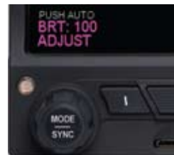
Figure 2-25 Display Brightness in BRT ADJUST Mode
