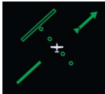
Figure 3-26 CDI Shown Hollow at Full-Scale Deflection
