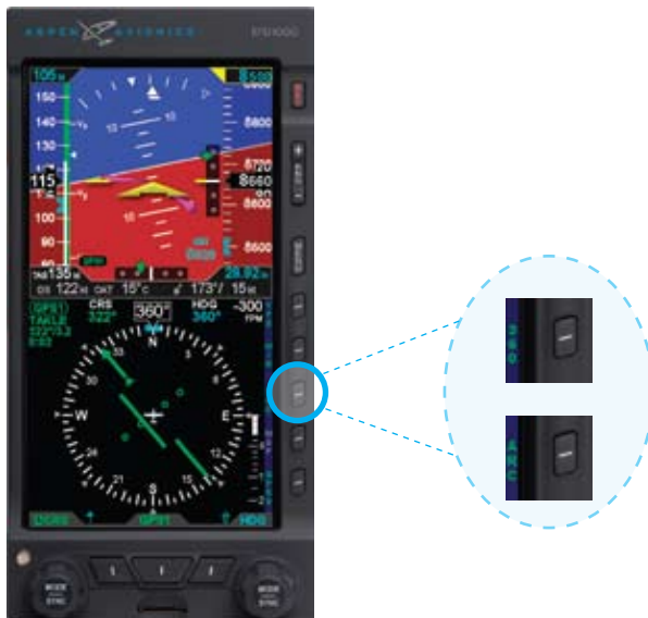
Figure 4-39 360/ARC Hot Key
