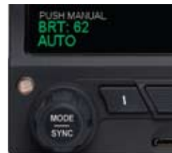
Figure 2-24 Display Brightness in BRT AUTO Mode
