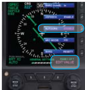
Figure 2-23 EDIT VALUE Displays Above Right Knob
