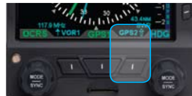
Figure 4-74 Double-Line Bearing Pointer and Button
