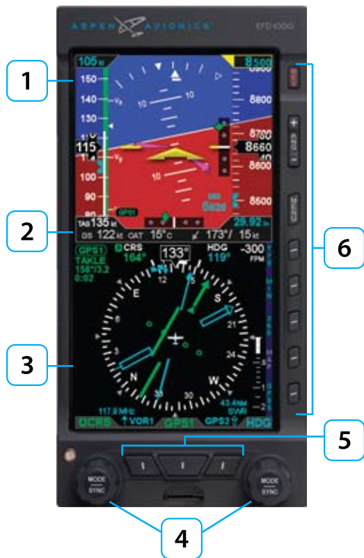
Figure 1 EFD1000 PFD Display, Knobs , Buttons, and Keys
