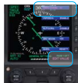
Figure 4-17 BARO Set to mB (millibars)
