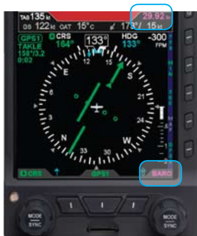
Figure 4-18 BARO Field Enabled
