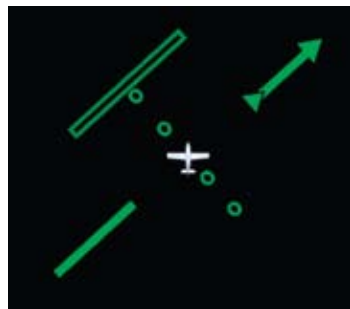
Figure 4-54 Exceeded Deviation, 360° and ARC HSI
