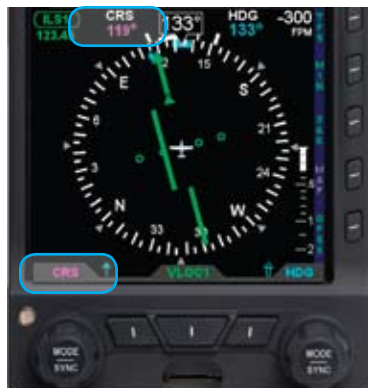
Figure 4-68 CRS Field Enabled for Editing
