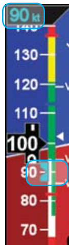
Figure 4-8 New Airspeed Selected
