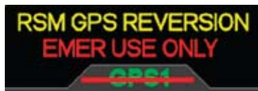
Figure 4-89 GPS1 Failure, Reversionary Navigation
