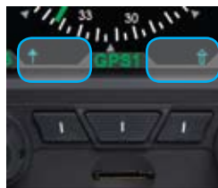
Figure 4-72 Bearing Pointers OFF
