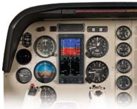
Figure 1-2 Single-tube EFD1000 PFD system
