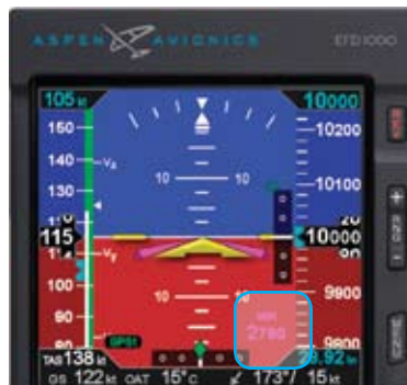
Figure 4-23 Selected Minimums Enabled
