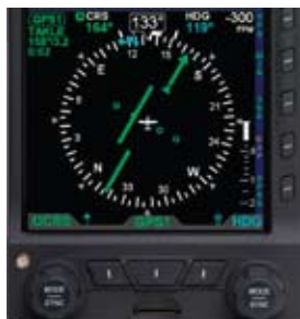
Figure 4-70 NO bearing pointers or source information
