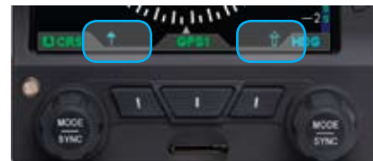
Figure 3-13 No Bearing Pointer Sources Selected
