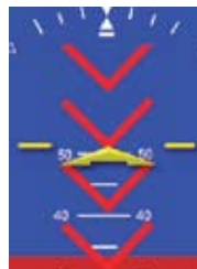
Figure 4-2 Pitch Markings - Large Pitch Down
