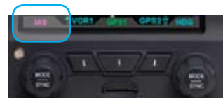
Figure 3-22 Selected Airspeed Bug Enabled
