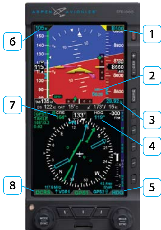
Figure 2-3 Left and Right Knobs and Corresponding Fields
