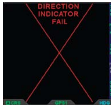
Figure 4-79 Direction Indicator Fail
