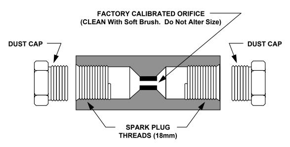
FIGURE 20-7. MASTER ORIFICE TOOL (For procurement, see chapter 2)
