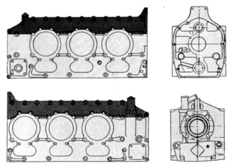
FIGURE 21-3. INSPECTION OF CRANKCASE CRITICAL (GRAY) AND NON CRITICAL (DARK GRAY) AREAS
