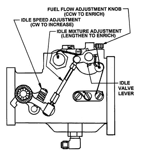
FIGURE 23-3. FUEL MIXTURE ADJUSTMENT
