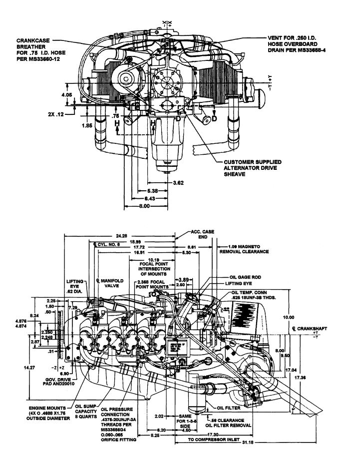
FIGURE 1-2. ENGINE DESCRIPTION L/TSIO 360-RB (Cont'd)
