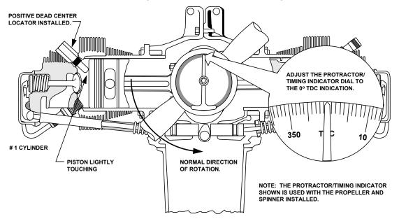
**FIGURE 12-4 TIMING POSITION STEP 1**
