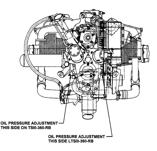
FIGURE 23-1. OIL PRESSURE ADJUSTMENT
