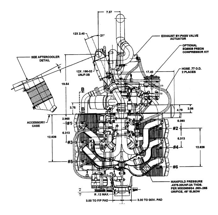
FIGURE 1-1. Engine Description L/TSIO-360-RB
