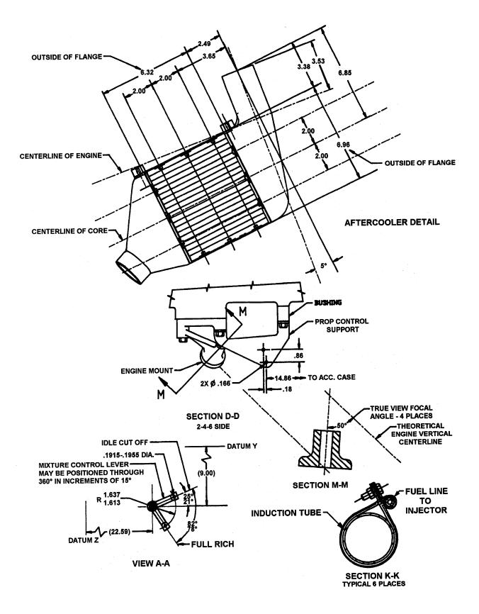
FIGURE 1-2. ENGINE DESCRIPTION L/TSIO 360-RB (Cont'd)
