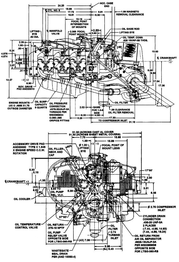
FIGURE 6-1. INSTALLATION DRAWING (cont'd)
