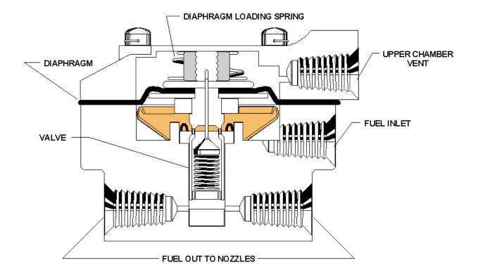
FIGURE 13-2. GENERAL FUEL MANIFOLD VALVE DESCRIPTION
