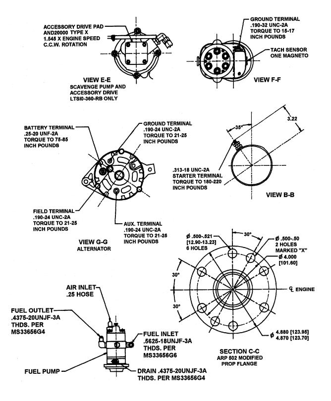
FIGURE 1-2. ENGINE DESCRIPTION L/TSIO 360-RB (Cont'd)
