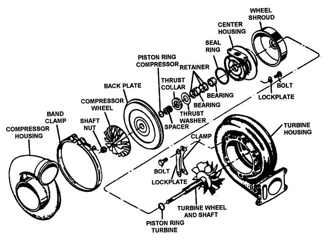
FIGURE 11-2. BASIC TURBOCHARGER
