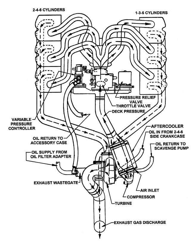
FIGURE 11-1. INDUCTION AND EXHAUST SYSTEM
