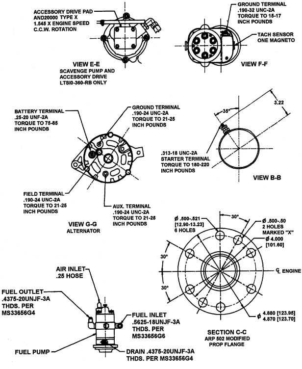
FIGURE 6-1. INSTALLATION DRAWING (cont'd)
