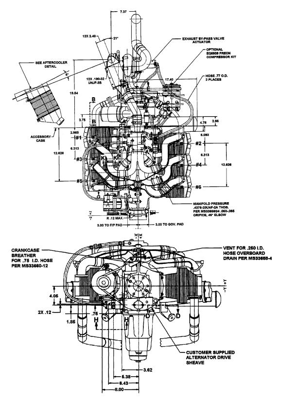
FIGURE 6-1. INSTALLATION DRAWING
