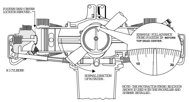
FIGURE 12-5. TIMING POSITION STEP 5
