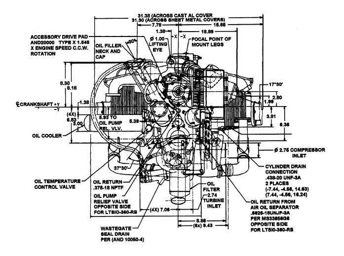
FIGURE 1-2. ENGINE DESCRIPTION L/TSIO 360-RB (Cont'd)
