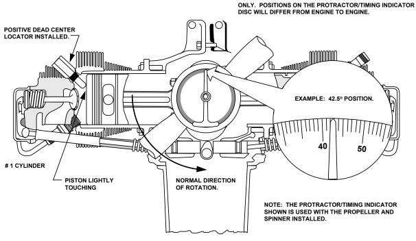
FIGURE 12-5. TIMING POSITION STEP 3
