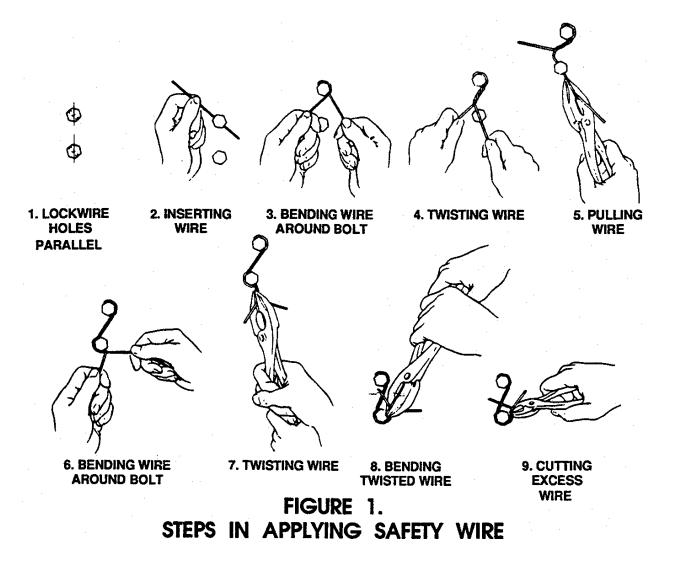
FIGURE 9-1. GENERAL LOCKWIRE PROCEDURE
