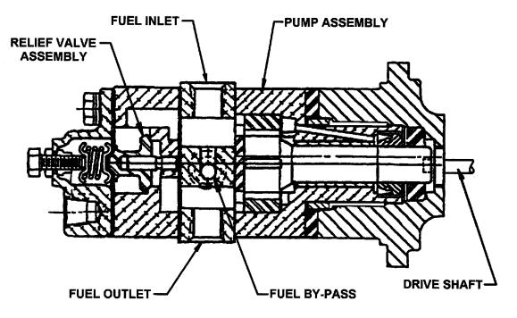
FIGURE 13-1. FUEL PUMP DESCRIPTION L/TSIO-360-RB
