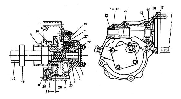
FIGURE 17-3. STARTER ADAPTER FITS AND LIMITS (LTSIO-360-RB and OPTIONAL TSIO-360-RB)
