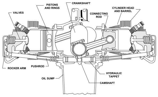
FIGURE 20-2. CYLINDER PISTON AND VALVE TRAIN
