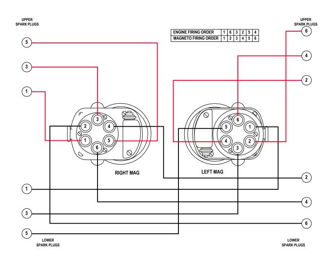
FIGURE 12-10. IGNITION WIRING DIAGRAM
