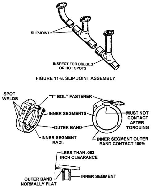
FIGURE 11-7. MULTI-SEGMENT "V" BAND CLAMP
