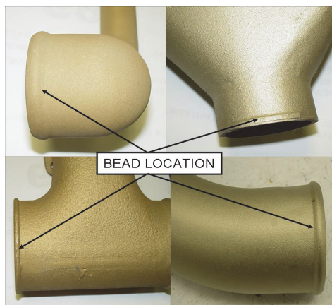
Figure 6-89. Induction Tube Bead Location
